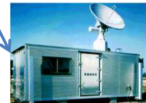
X-band Research Doppler Radar (9.8 GHz) MRI, JMA, 1982
